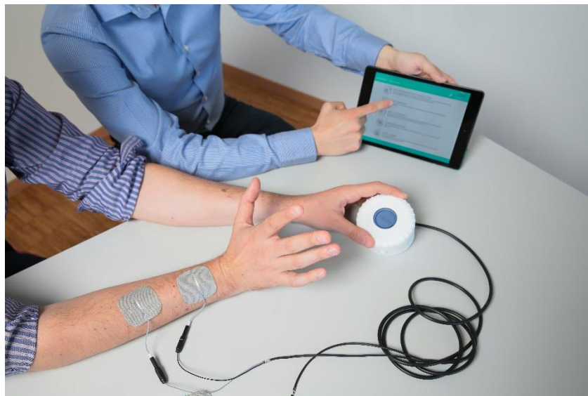
The system is composed by a tablet application and controller device meant to be used with the healthy hand of the patient. © 2017 Alain Herzog
